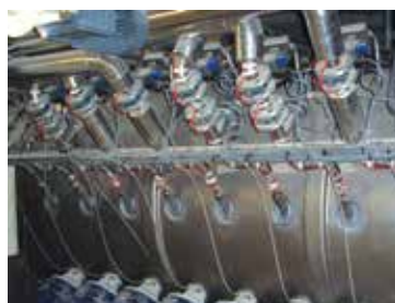
Choppers, liquid injectors, temperature jacket
